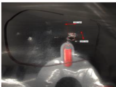
Picture 2: Cut through the film and a few notches in film surface
