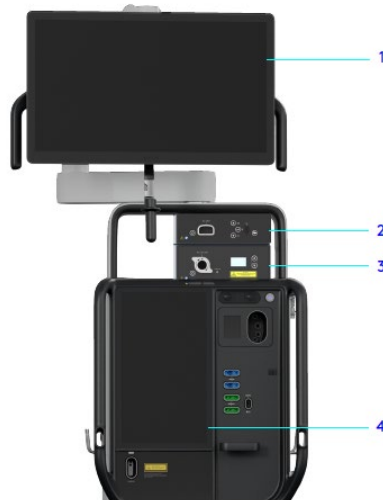
Figure 4. Placement of CCU and light source (example)
