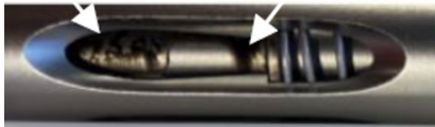
Figure 1: Heterogeneous coating of the Pin Chuck
