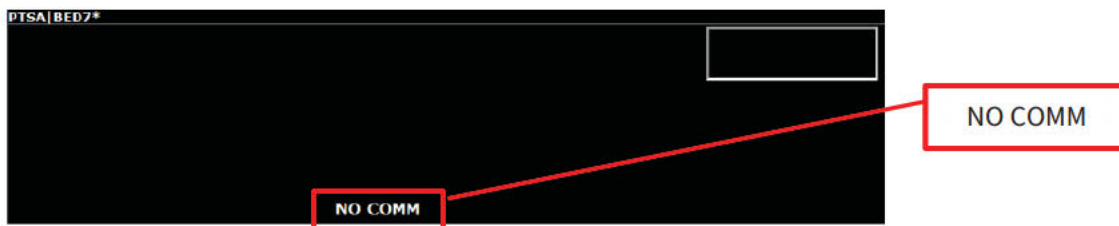
Figure 1. NO COMM condition example in the Central Station Multi-Viewer window with no audible or visual alarm indicators.
