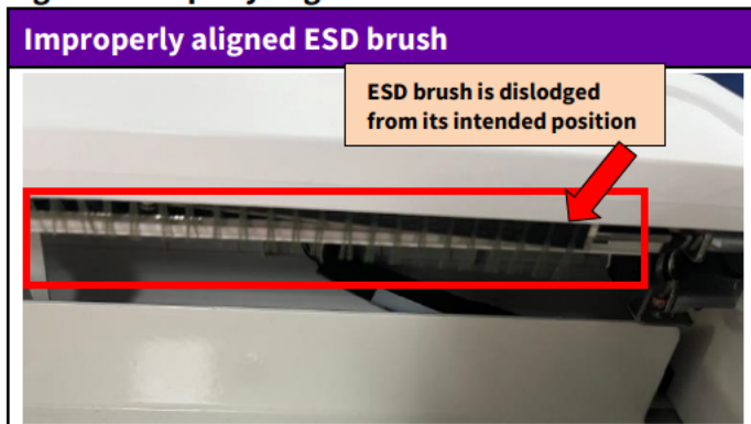
Figure 2: Improperly aligned ESD brush
