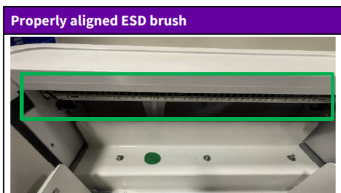
Figure 1: Properly aligned ESD brush.
