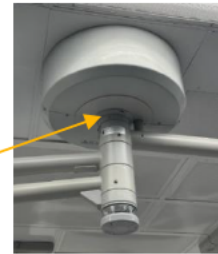
Image 1: Affected Component: Soffit Ring
