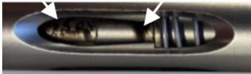
Figure 1: Heterogeneous coating of the Pin Chuck
