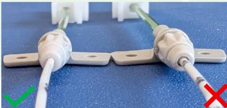
Figure 1: Comparison of the gap dimensions between the correct screw nut (left) and the faulty screw nut (right)
