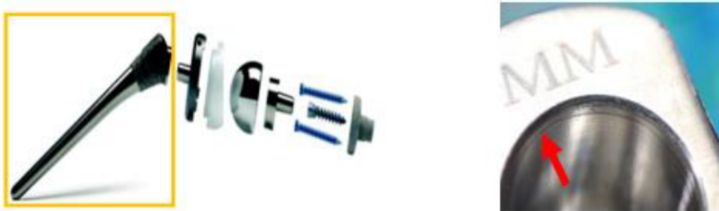
Figure 1 – The Comprehensive Shoulder Primary Stem (left) did not fit properly due to excess metal that was identified on the inner taper (right).
