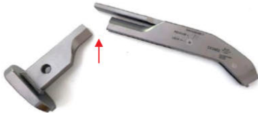
Figure 3: Broken universal handle 130-394/01.
