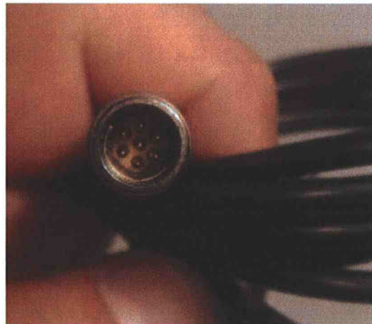
Figure 5: Connector of HL 40 Bubble Sensor (Article no. 701065317)
