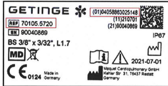
Figure 3: Type label with incorrect UDI 04058863025148
