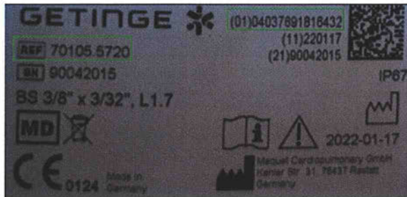
Figure 2: Type label with correct UDI 04037691816432
