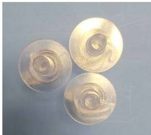
Figure 2: Incorrect filter connectors with occluding fleece
