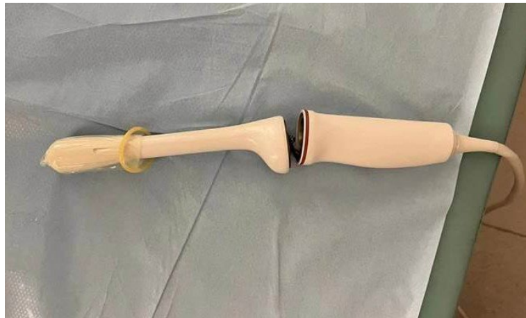
Figure 1. Transducer Bond Failure
