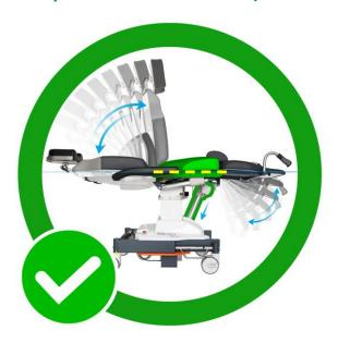
**ATTENTION!** The seat part must be in a horizontal position to the floor (see green cushion), the seat part drive remains in the retracted position (green marked component). Adjustment movements, e.g. into the reset position, are still possible (see adjustment positions of back and leg part shown in grey).
