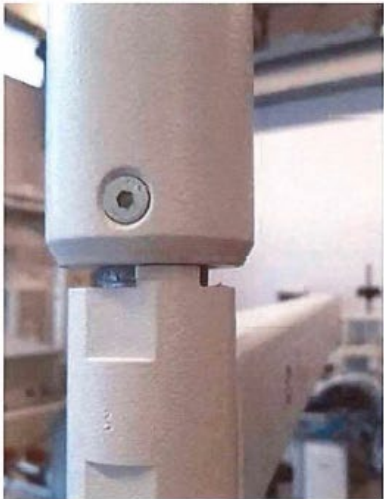
No gap, system is not affected - OK
