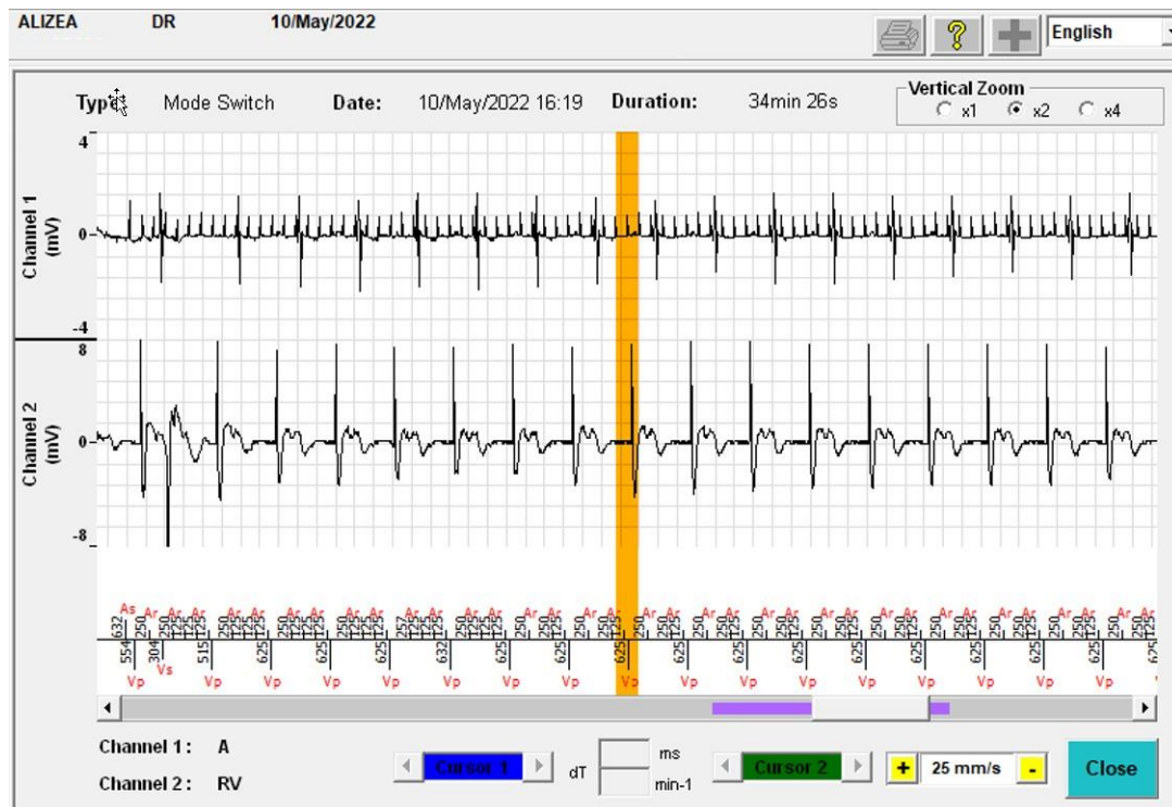
Figure 3: Illustration of “Mode Switch” episode due to MV noise oversensing on a DR pacemaker
