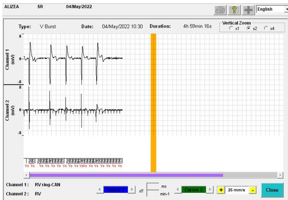
Figure 2: Illustration of “V Burst” episode due to MV noise oversensing on an SR pacemaker
