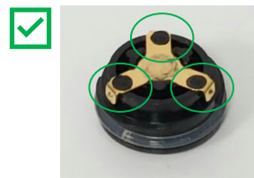
Undamaged battery cap - Continue to use Has three raised, round, black, plastic dots holding metal contact in place
