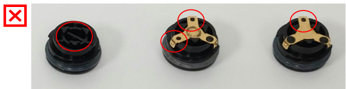
Damaged battery caps - Do not use Metal contact is missing, or fewer than 3 raised
