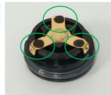
Undamaged battery cap - Continue to use Has three raised, round, black, plastic dots holding metal contact in place
