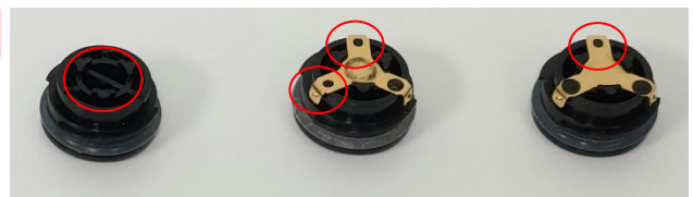
Damaged battery caps - Do not use Metal contact is missing, or fewer than 3 raised
