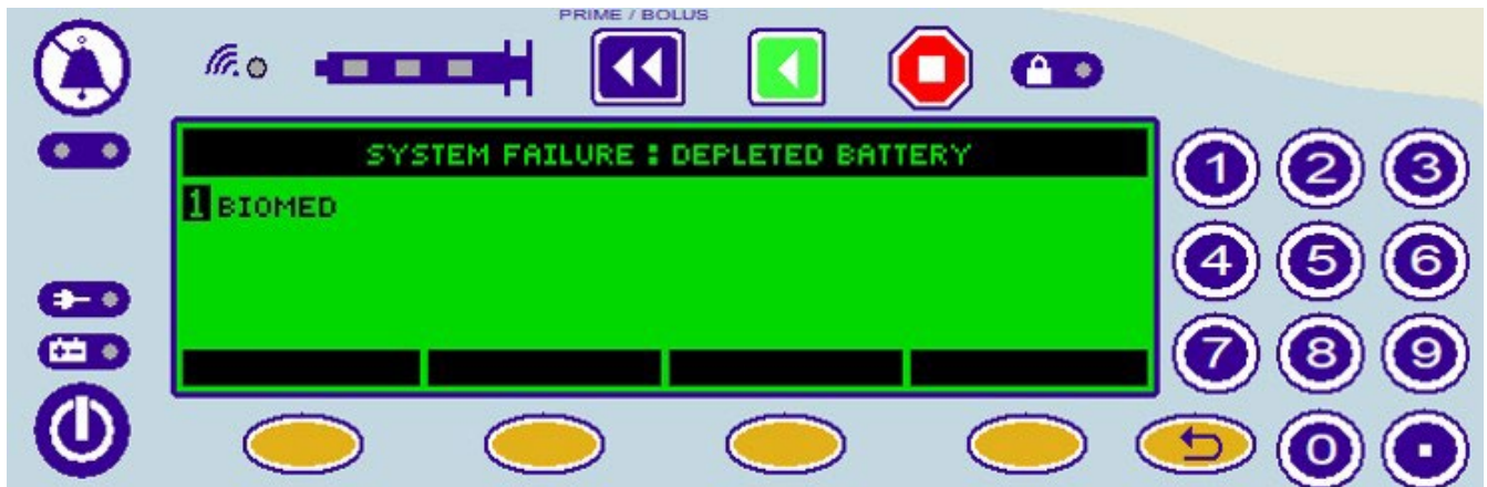
Figure 1: System Failure: Depleted Battery Alarm
