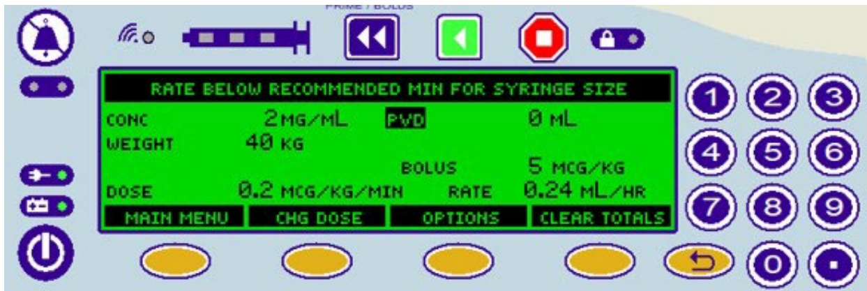
Figure 3: False Rate Below Recommended Minimum for Syringe Size Alarm
