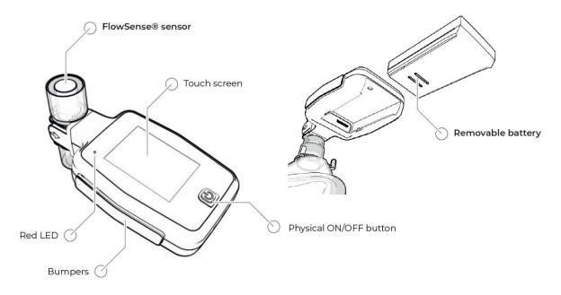
EOlife® is connected with the FlowSense® sensor which is placed between a ventilation interface (mask or probe) and a standard self-inflating bag for manual ventilation of the adult patient.
