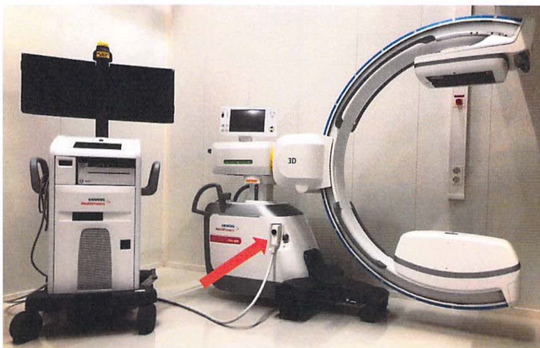
figure 1: example of X10 connector with main cable, connected to Cios Spin c-arm
