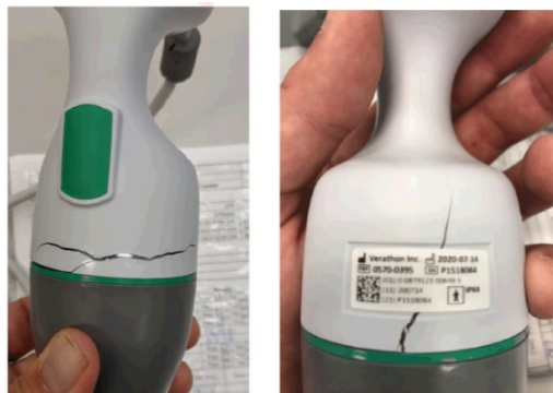
Figure 1: Example of cracked probe handle
