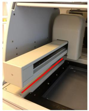
Visually inspect the left plate, area highlighted in red, for signs of unexpected leakage (salt residues and/or liquid). This might indicate leakage from the robotic arm.
