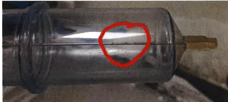
Figure 2: Halo on the stainless-steel needle inside the rigid chamber, component H
