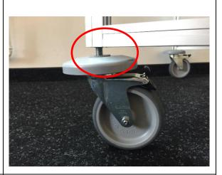
**Tightening the screw** connection with hex key (wrench size: 6 mm)
