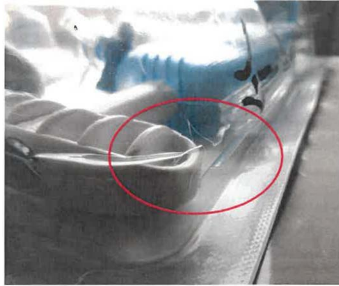
Picture 1 : Example of crack observed near the DOLPHIN inflation device handle
