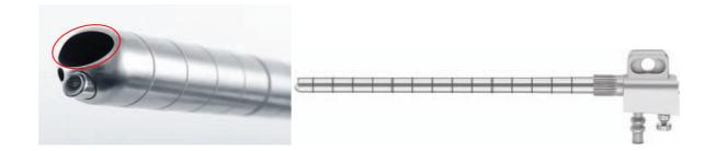
The initiated investigation showed that the distal working end of the trocar was not clear from burrs. The failure was caused by a deviation in the production process which could be traced back to a limited period of time. There is a possibility that other MINOP INVENT TROCARS, FH620R, which were manufactured during that period of time might also be defective.
